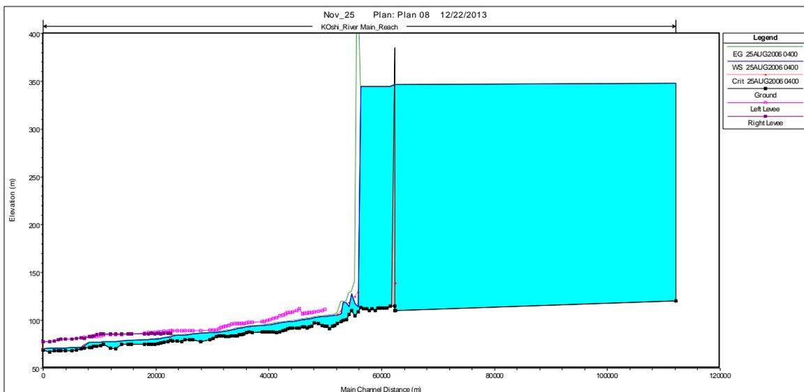
c. Profile during the breach (Intermediate)
