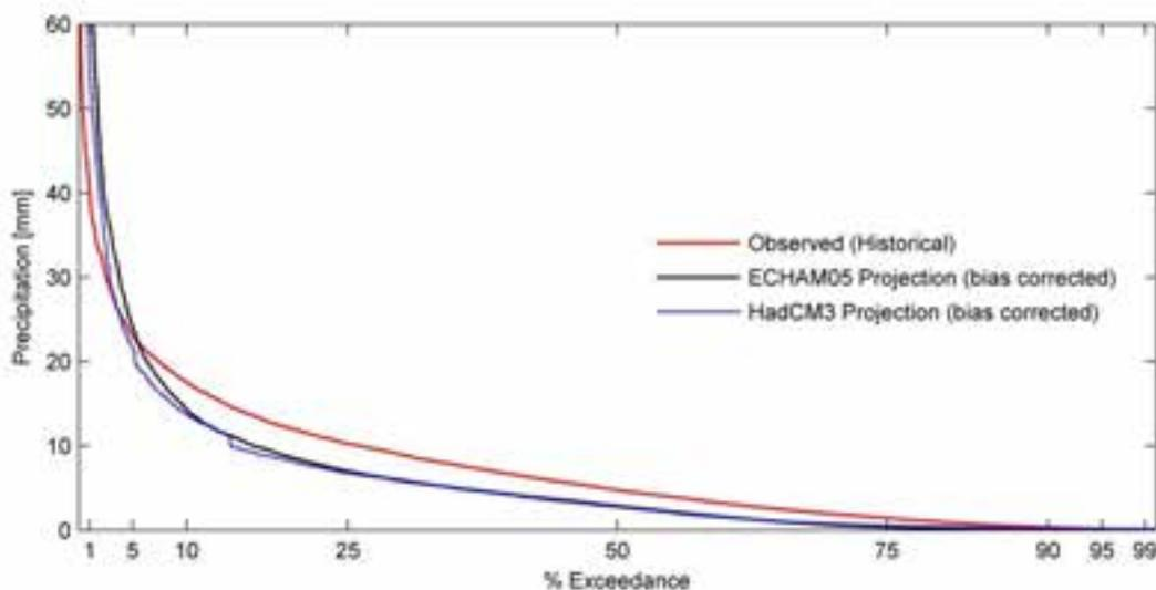
**Figure 5-16: Percentage Exceedance graph for precipitation values from historical and bias corrected RCM data sets for the SWAT model area**
