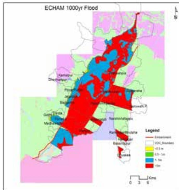
Figure 8-7: Inundation under 1000 year ECHAM05 flood
