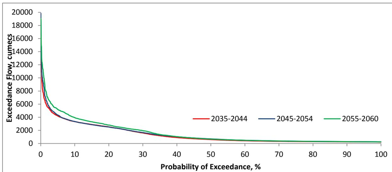
Figure 7-22: Decadal Flow Duration Curves for Projected Series
