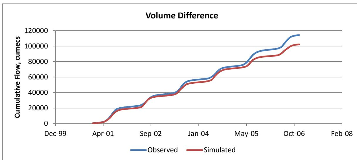
Figure 7-9: Comparison of Observed and Simulated Volumes
