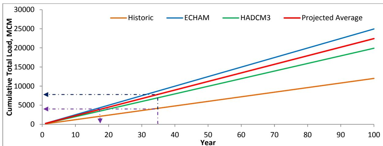
**Figure 7-27: Sediment Load Estimates for different design years**
