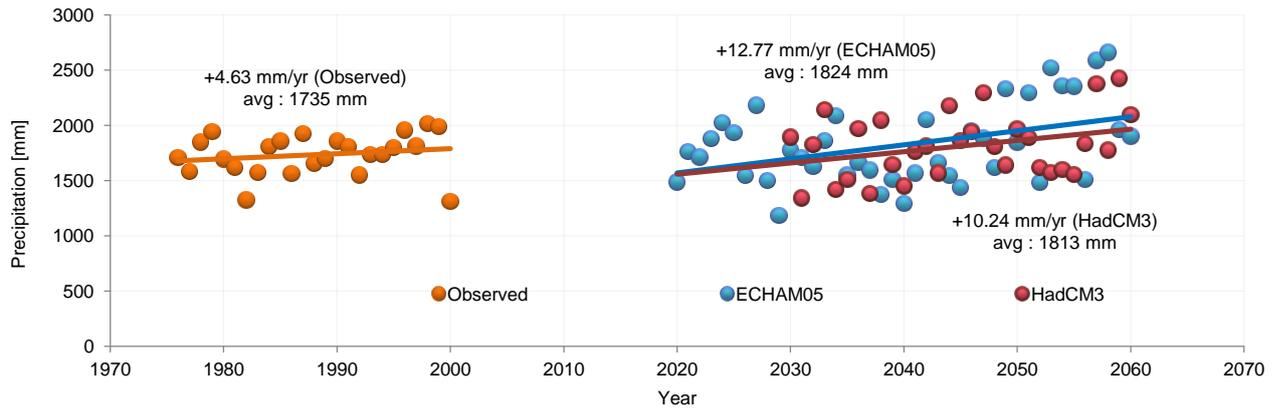
**Figure 5-15: Basin averaged annual precipitation comparison between historical and RCM projected data (including trend and average values) for the SWAT model area**
