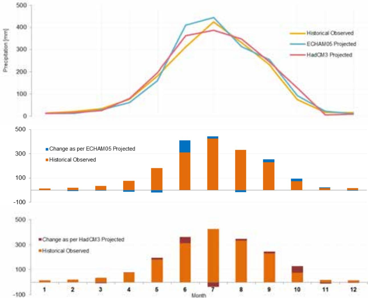
**Figure 5-14: Top: Basin averaged average monthly rainfall values for the SWAT model area for historical/ observed data and the RCM data. Middle: Change in the average monthly precipitation values from the observed data for ECHAM05. Bottom: Same for HadCM3**
