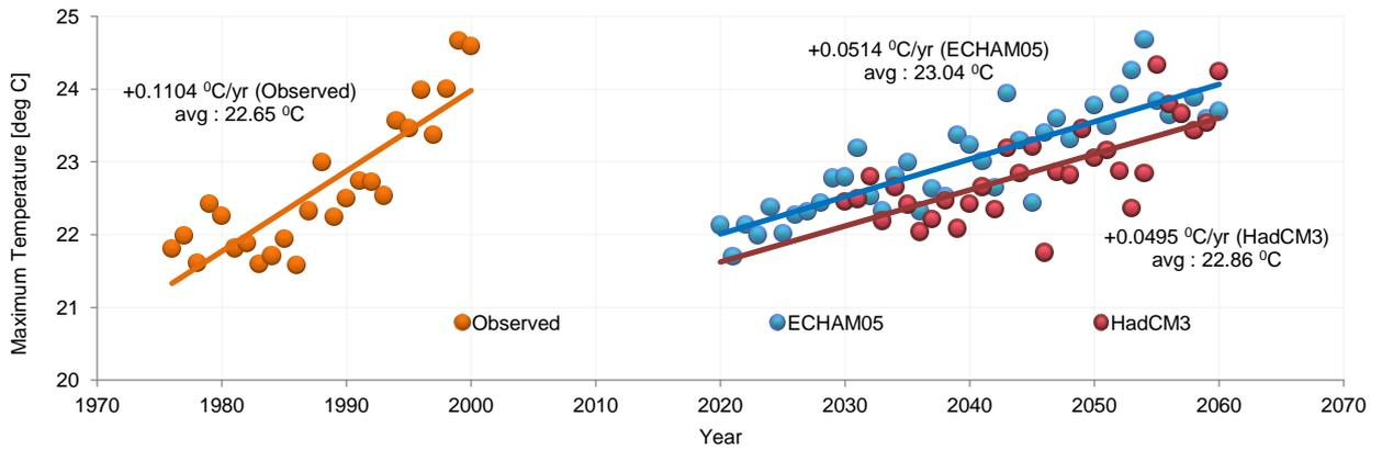
**Figure 5-19: Basin averaged annual average maximum temperature comparison between historical and RCM projected data (including trend and average values) for the SWAT model area**
