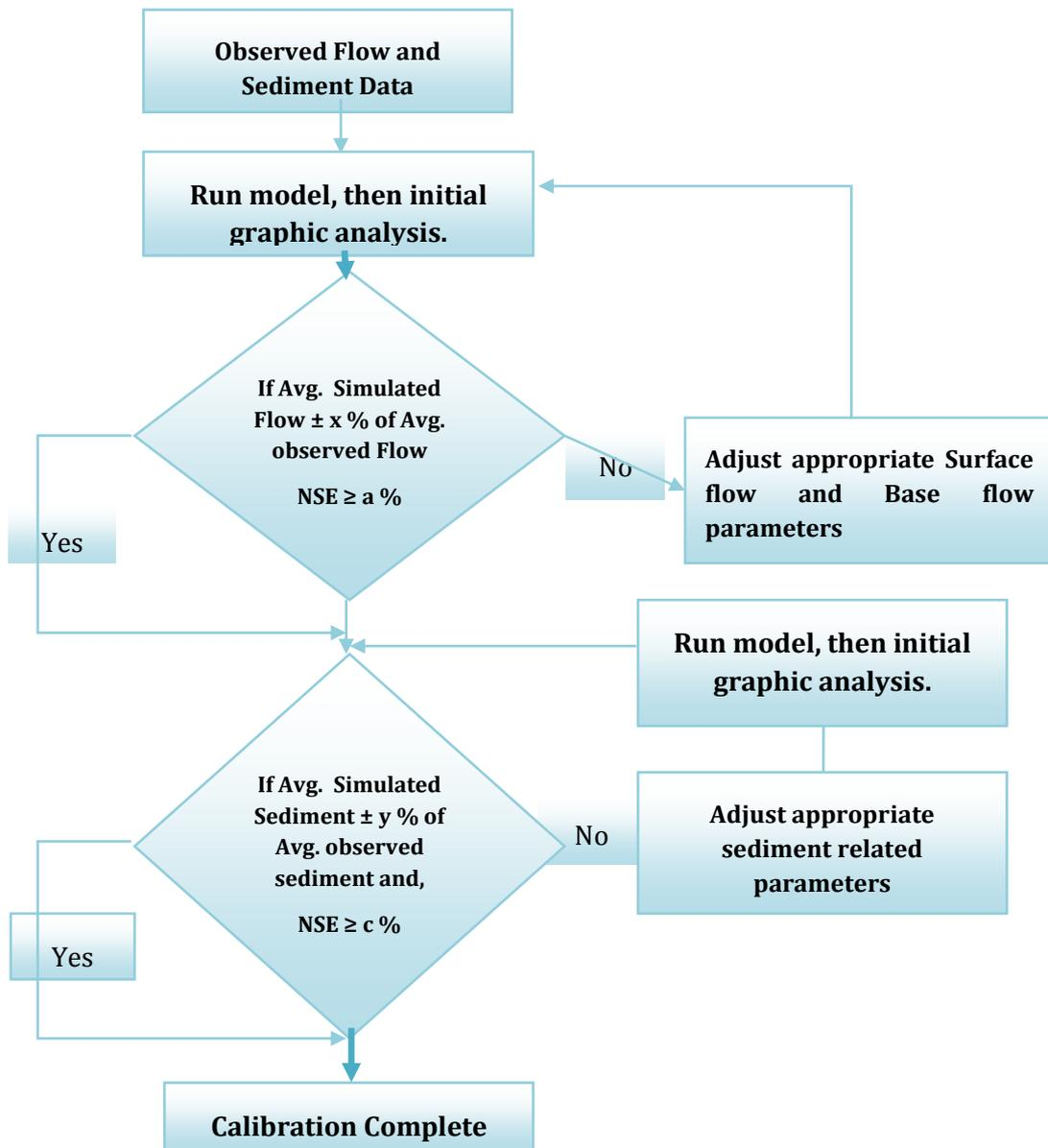
Figure 3-4: Calibration Process
