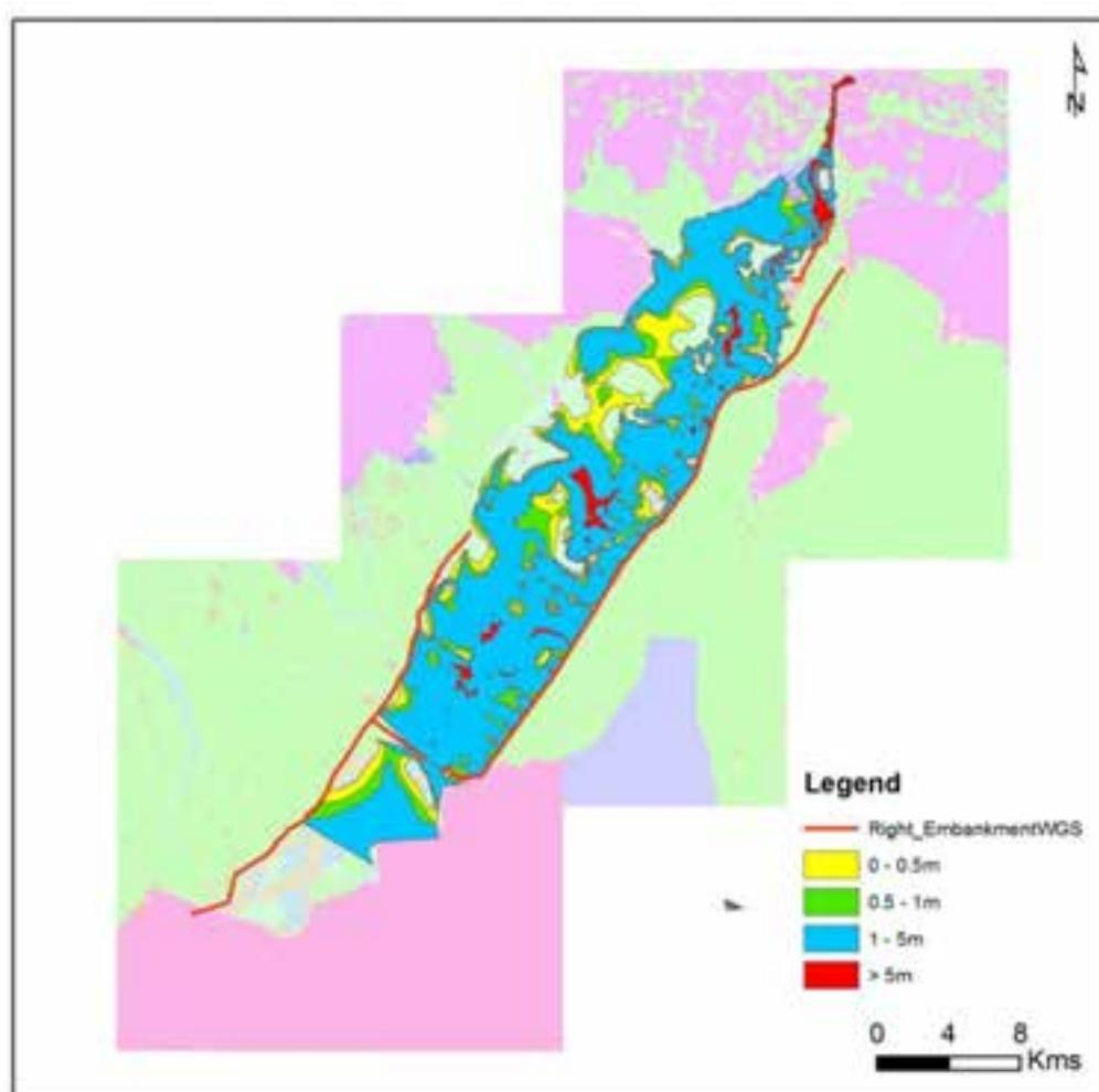
**Figure 8-4: Inundation Pattern under 100 yr Return Period Flood**
