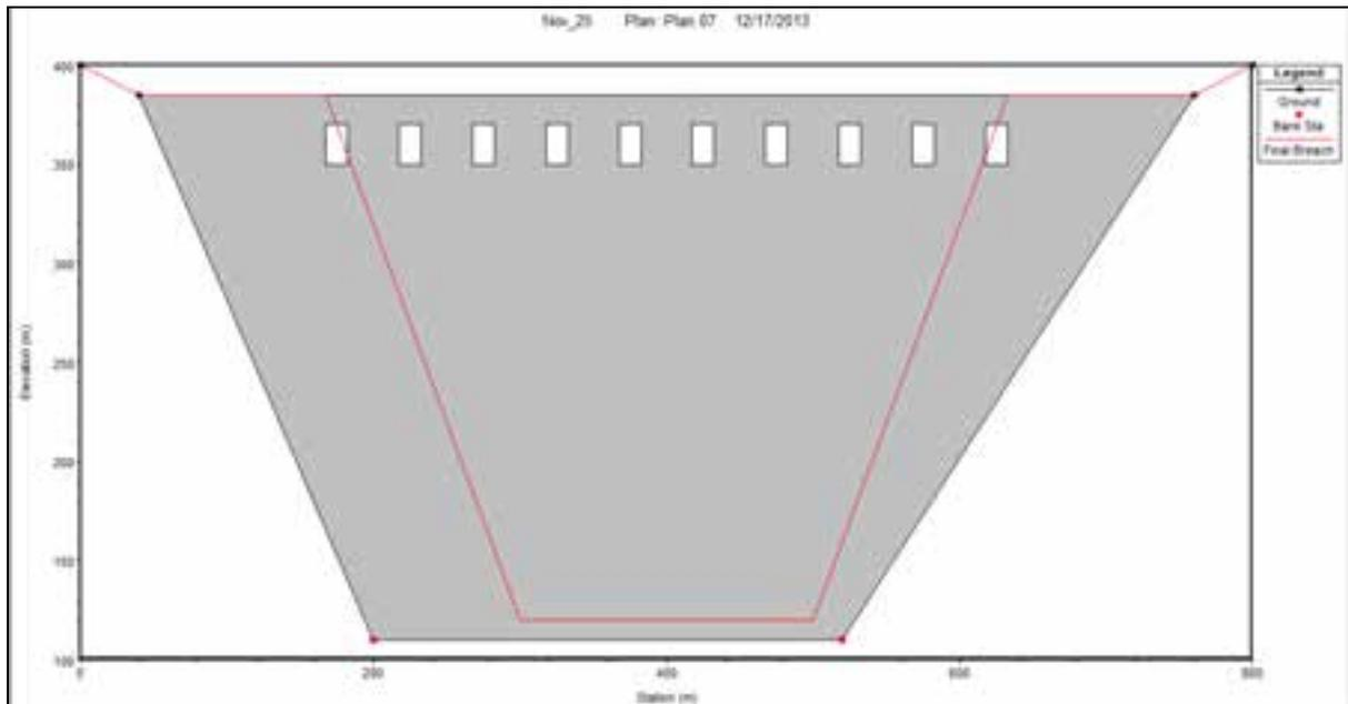
**Figure 8-11: Specification of the Breach**
