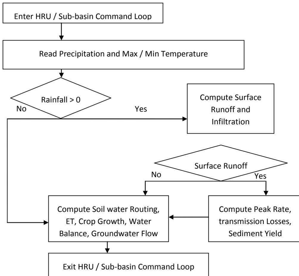
**Figure 3-3: HRU / Sub-Basin Command Loop**
