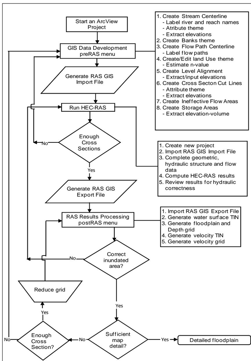
**Figure 3-5: Flow Chart for the Calculation of Flood Inundation**
