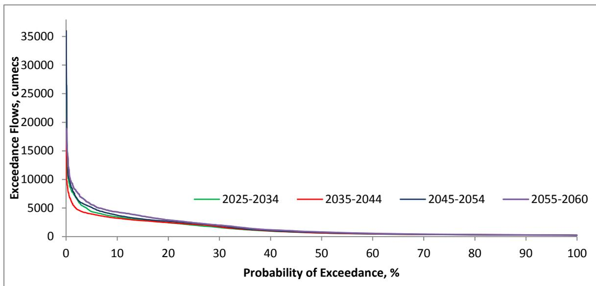
Figure 7-17: Decadal Flow duration Curves for Projected Series
