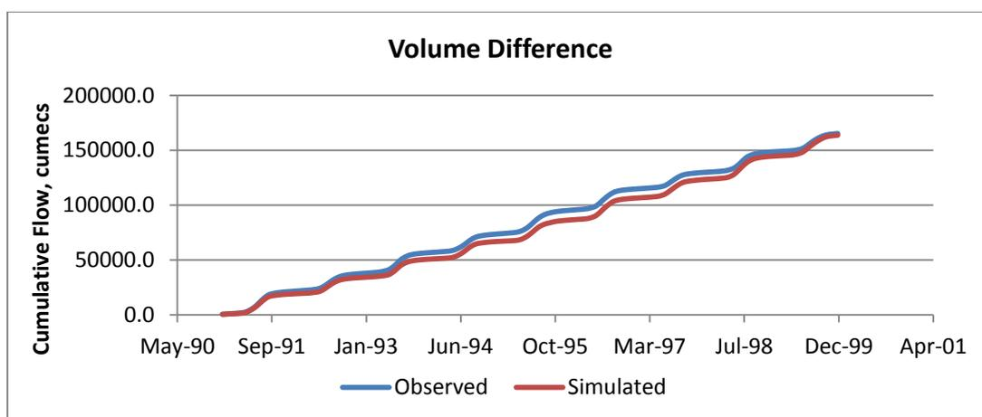
Figure 7-7: Comparison of Observed and Simulated Volumes
